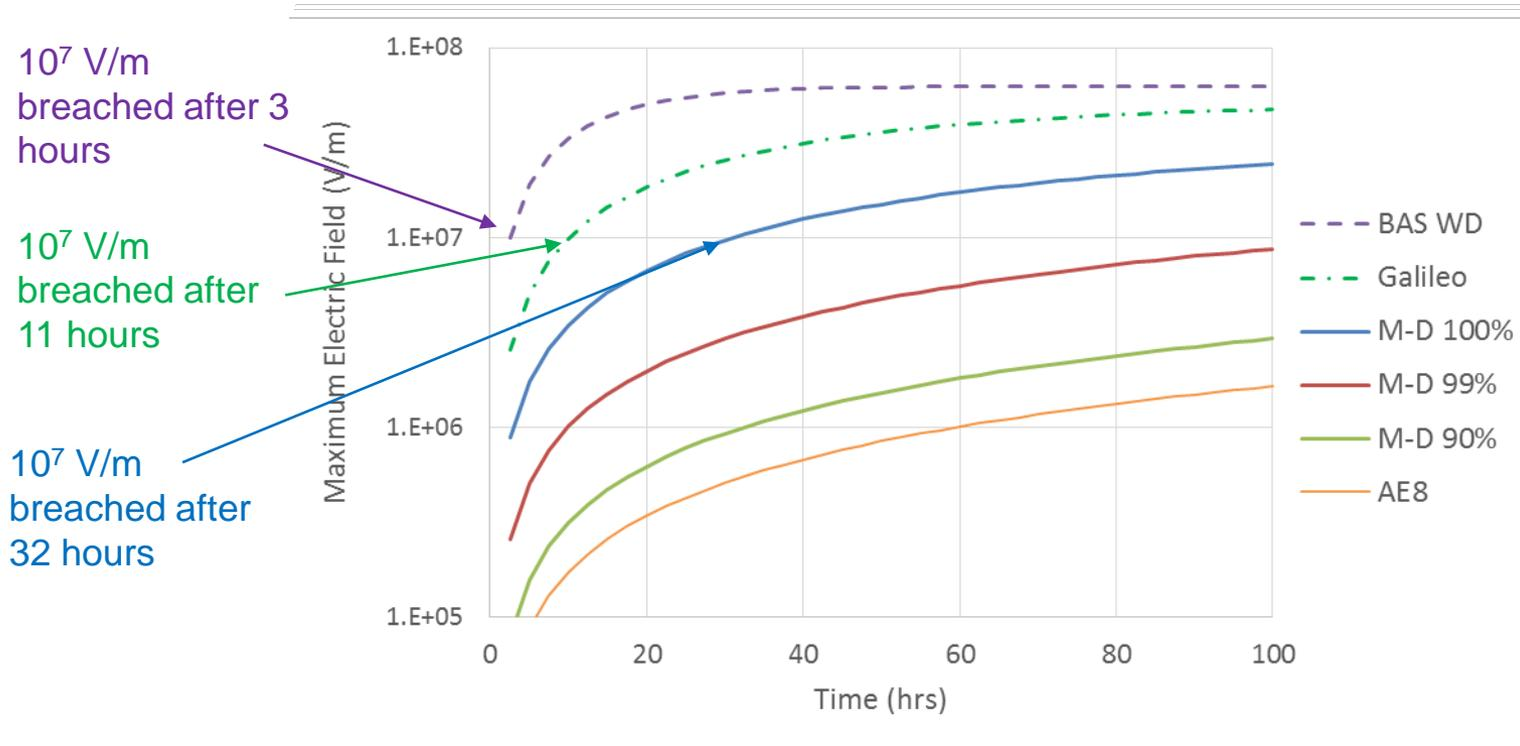
(NB rule-of-thumb estimate for electro-static discharge is  $10^7$  V/m)
