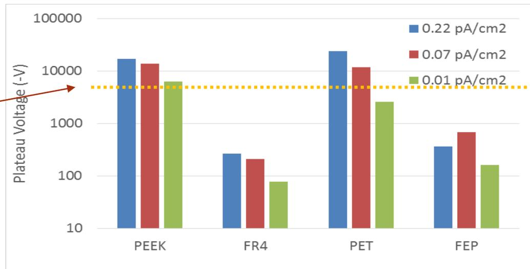
Critical Electric field threshold ( $\sim 10^7$  V/m) exceeded even at  $0.01$  pA/cm<sup>2</sup>
