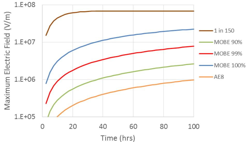
(NB rule-of-thumb estimate for electrostatic discharge is  $10^7$  V/m)
