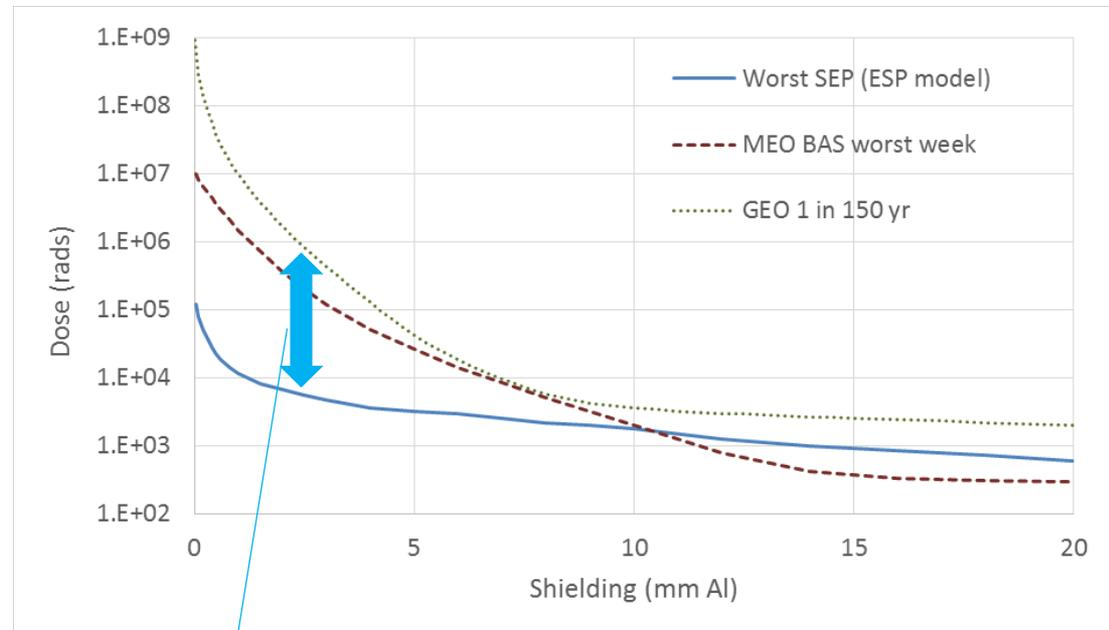
Electron worst case >> proton worst case up to relatively high shielding levels
