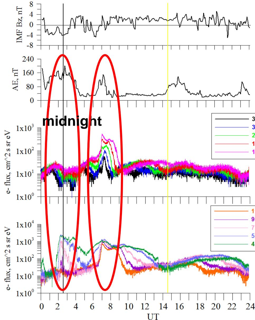
**The data:** AMC 12 geostationary satellite, CEASE-II (Compact Environmental Anomaly Sensor) instrument with Electrostatic Analyzer (ESA) for measuring low energy electron fluxes in 10 channels, 5 - 50 keV.
