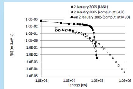
IMPTAM modeled electron fluxes are in a good agreement with LANL MPA and SOPA measurements at GEO. The maximum flux of 1-100 keV electrons of an order of magnitude larger than that observed at GEO was detected at MEO at 06 MLT after 2 hours from the surface charging event detected at GEO by LANL.
