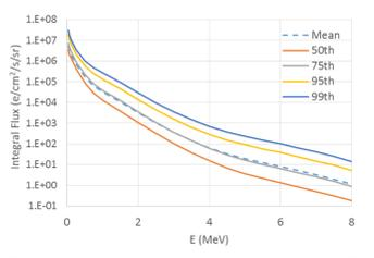
Figure 2: AE9 static mean percentiles for integral flux at GEO.
