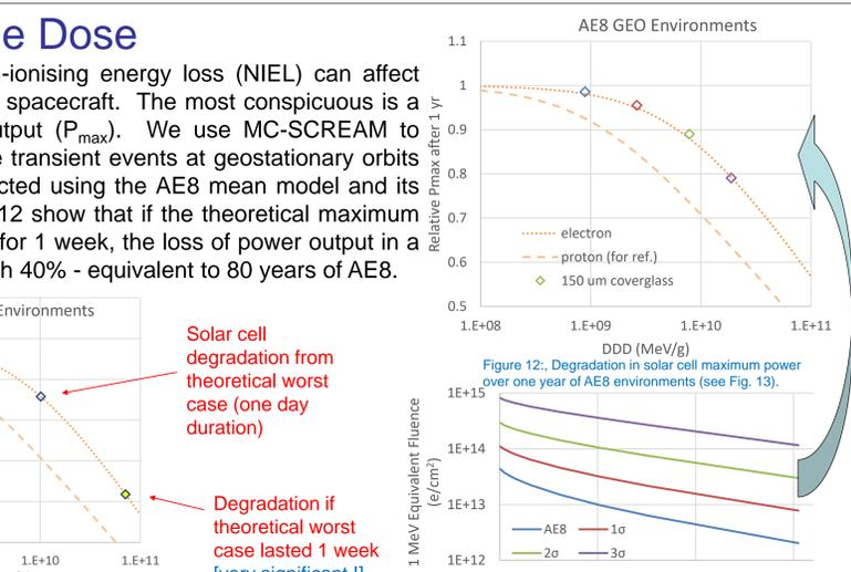
Figure 12: Degradation in solar cell maximum power over one year of AEB environments (see Fig. 13).
