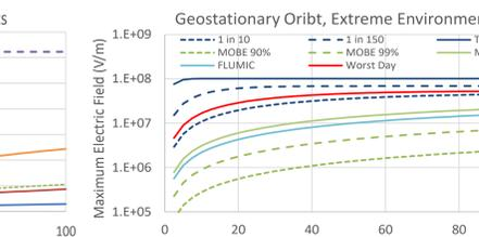
Figure 15: Charging profile of 1 mm PEEK sample under various models of electron enhancement at GEO. A typical breakdown threshold is 10<sup>7</sup> V/m.
