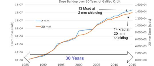
Figure 10: Cumulative Dose from reconstructed data set at two shielding depths.
