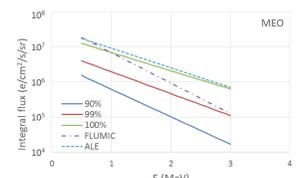
Figure 3: MOBE-DIC and FLUMIC electron spectra (including "Anomalous Large Event") at L=4.7.
