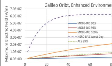
Figure 14: Charging profile of 1 mm PEEK sample under various models of electron enhancement at MEO. A typical breakdown threshold is 10<sup>7</sup> V/m.
