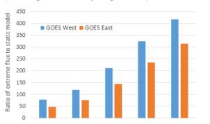
Figure 4: Enhancement factors of extreme events with respect to >2 MeV flux in AE8 static model.
