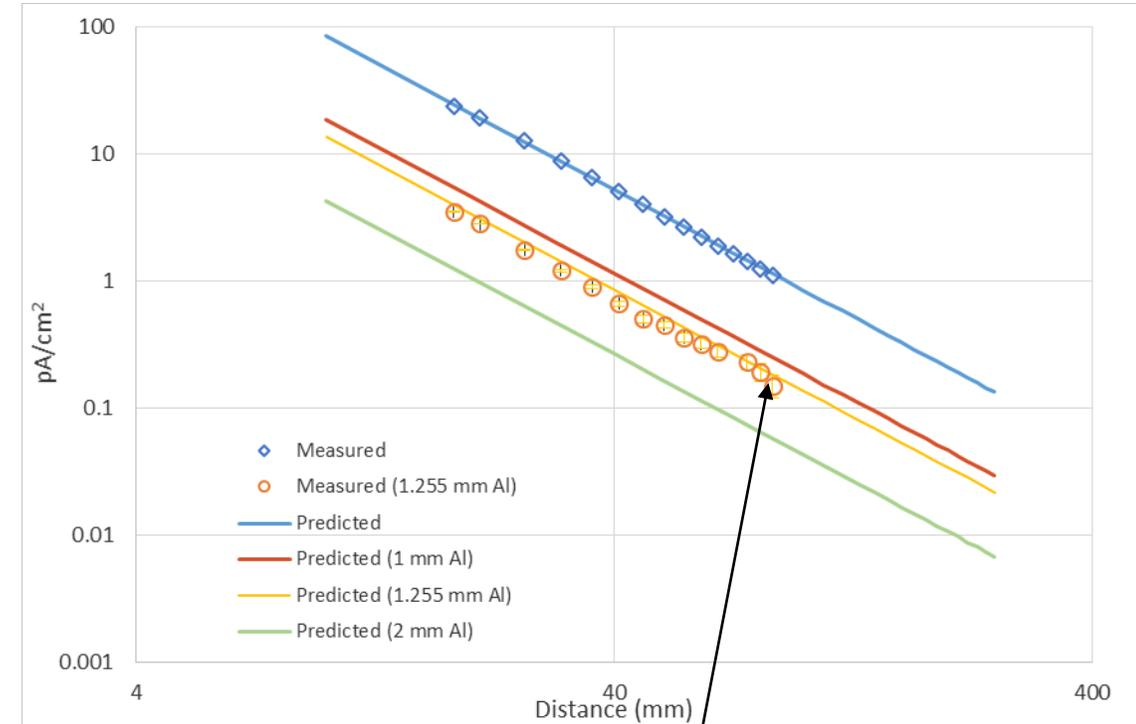
Shielded measurements consistent with simulations
