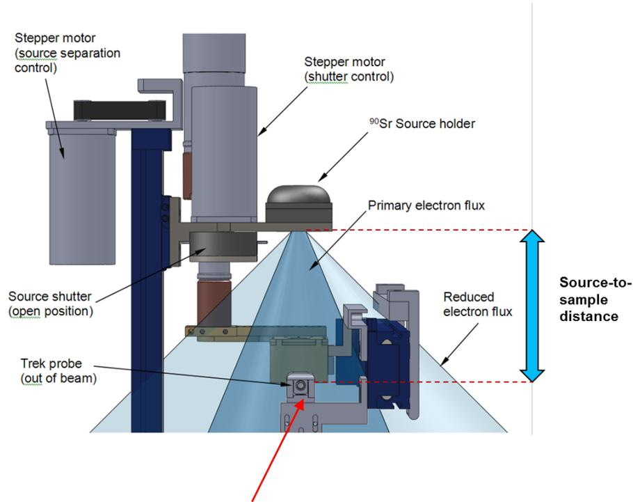
(Surface potential measured with non-contact Trek probe)
