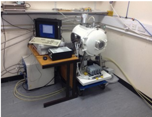
Realistic Electron Environment Facility (REEF) (Sr-90 source)
