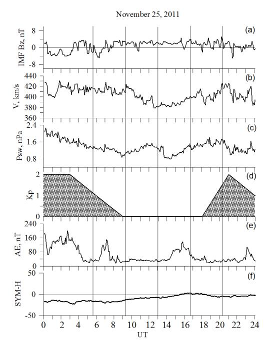
No storm is needed for 2-3 orders of magnitude increase of low energy electron fluxes at geostationary orbit
