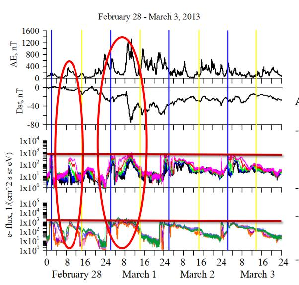
Small, CIR-driven storm with **Dst of 75 nT, IMF Bz** of -5 -10 nT, **Vsw** from 350 to 650 km/s, **Psw** peak at 8 nPa, **AE** peaks of 800-1200 nT
