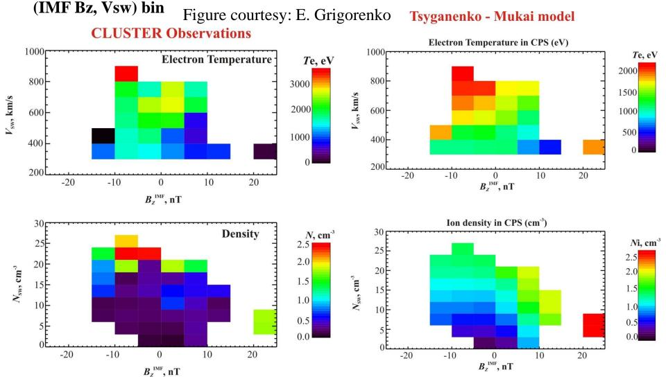
Measured electron temperature and number density different than those given by TM03 model
