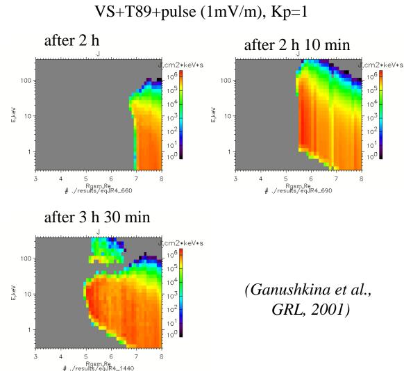
fast earthward shift of previous population by **impulsive electric field** associated with substorm dipolarization, 2 Re for about 1 hour,
