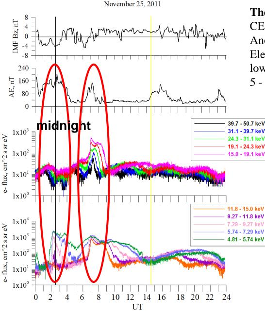
**The data**: AMC 12 geostationary satellite, CEASE-II (Compact Environmental Anomaly Sensor) instrument with Electrostatic Analyzer (ESA) for measuring low energy electron fluxes in 10 channels, 5 - 50 keV.
