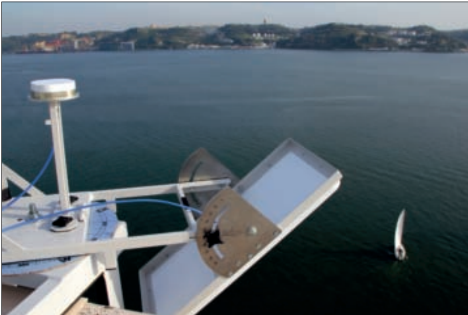
Ground based GNSS-Reflectometer testing campaign in the Tagus river.
